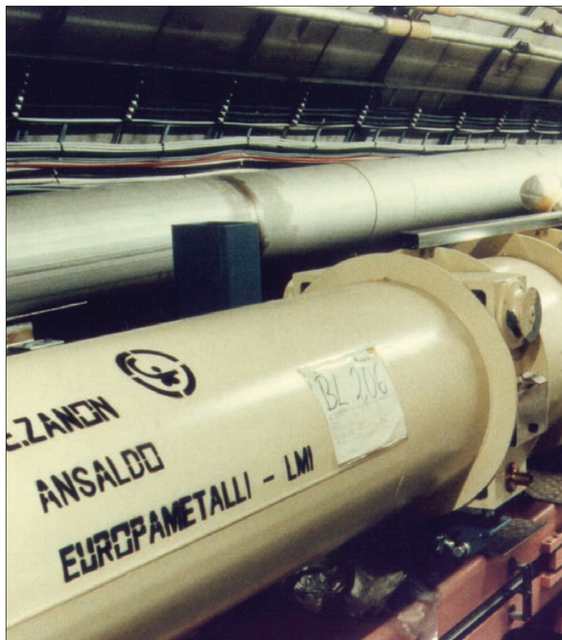
Inside the HERA tunnel: the proton accelerator with its superconducting magnets (be
