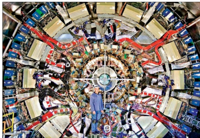
The cryostat flange of the ATLAS barrel showing the material added by services (cables, pipes and protections). (Courtesy H Pernegger/CERN.)
